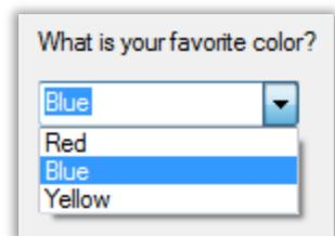
You will find the list box and combo box controls in the Toolbox under "Common Controls" just like the text box. Follow the same drag-n-drop procedure to add either control to your form.
