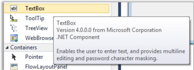
To add this control to your form, you can double-click it in the Toolbox or click and drag it from the Toolbox to the Form Design screen. You can click on the control’s outline and then drag the mouse to resize or move the text box on the form.
